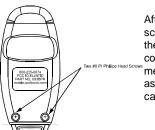
After removing the two #0 point phillips screws shown pry apart case with the edge of a finger nail or a small common screwdriver. Keep hold of the metal key ring loop to prevent it's loss as it will separate from the transmitter case.
